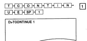
Input the TCONTINUE command and a task number (AD51H-S3: 1 to 8, A1SD51S: 1, 2) to resume a BASIC program stopped by the TSTOP command. (This example assumes that task No.1 is designated.)
